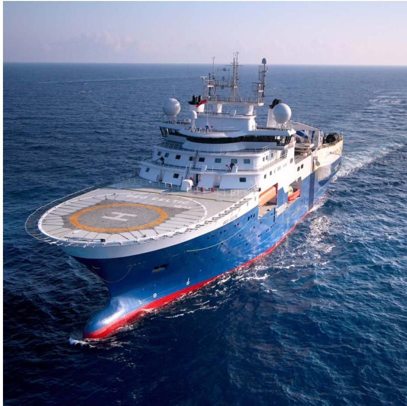
Figure 1 - Geo Celtic 3D seismic survey vessel
